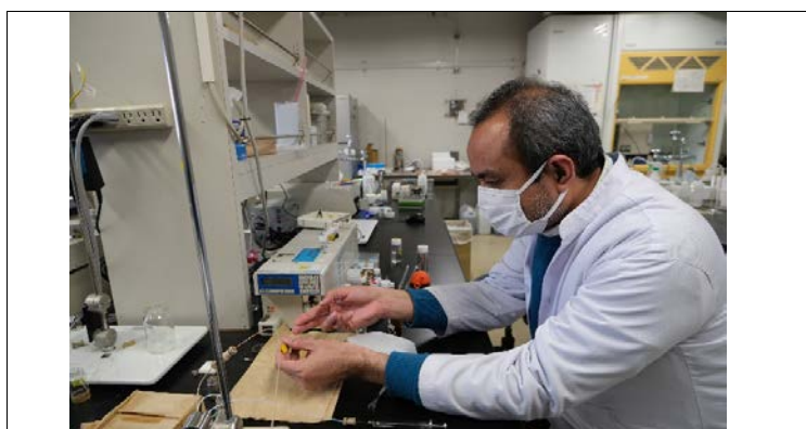
Installing the column on the capillary liquid chromatography apparatus
