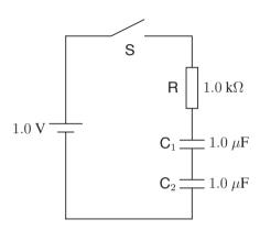
Q4 What is the quantity of Joule heat (in  $\mu$ J) evolved at R from when S is closed until C<sub>1</sub> and C<sub>2</sub> become fully charged? From ①-④ below choose the best answer.
