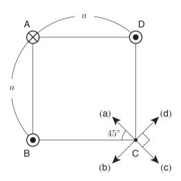
Q5 What is the magnitude (denoted as H) of the magnetic field produced at C by the currents flowing through the three wires? Also, which arrow among (a)-(d) in the figure indicates the direction of that magnetic field? From ①-(8) below choose the correct combination.
