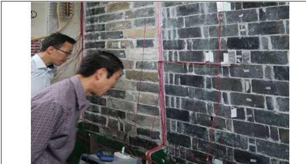
吸水実験/Water absorption experiment
