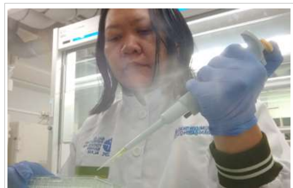
Testing the antioxidant activity of the extract using microplate 96 well
