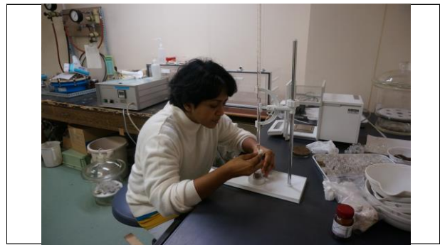
土壌の撥水性測定/water drop penetration time
