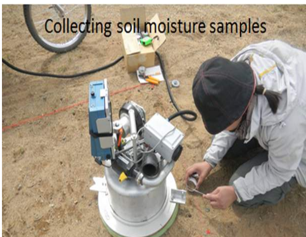
Measuring dust emission using a mini wind tunnel and collecting soil moisture samples 2009.May / Mongolia
