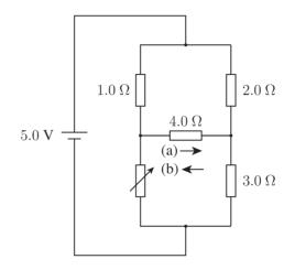
Q4 When the resistance of the variable resistor is set as  $0 \Omega$ , does the electrical current flowing through the 4.0- $\Omega$  resistor flow in the direction of arrow (a) in the figure, or in the direction of arrow (b)? Also, at what resistance setting of the variable resistor will the current stop flowing through the 4.0- $\Omega$  resistor? From (1)-(4) below choose the best combination. **16**
