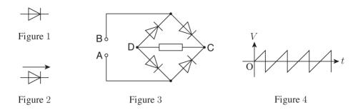
Q5 If current flowing in the direction from C to D in the figure is defined as positive, how does current *I* flowing through the resistor change over time t? From ①-⑧ below choose the graph that best represents this change. **17**
