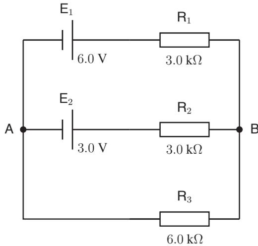
**Q3** What is the magnitude of the electric current flowing through resistor  $R_2$  (in mA)? Also, is the direction of the current from **A** to **B**, or from **B** to **A**? From ①-⑥ below choose the best combination.
