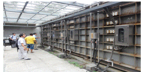
土壌における重金属遷移実験装置(中国環境科学研究院)/Experiments for heavy metals migration in soil. (Chinese Research Academy of Environmental Sciences)
