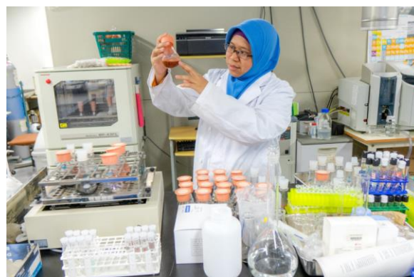
振盪機を用いた金浸出実験 / Gold leaching test using shaker equipment
